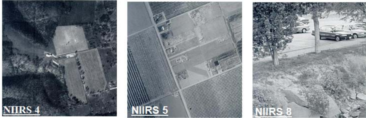
Fig. 1. Sample overhead imagery and its corresponding NIIRS ratings illustrate the level of image analysis tasks that could be supported. Description of NIIRS level criteria are provided in the text above.
