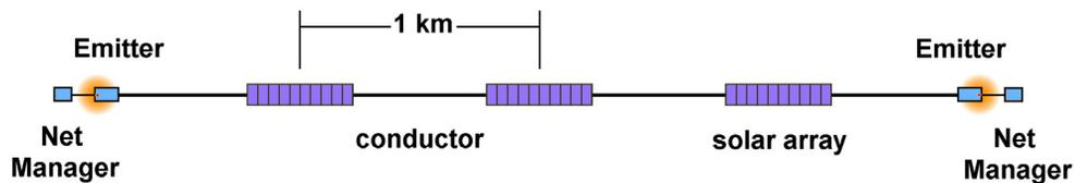
Fig. 2. Representative Sections of the 10-km-Long EDDE Vehicle.
