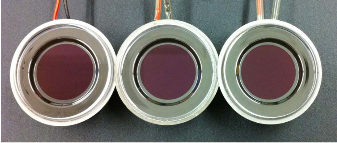
Fig. 3. 18 mm anode sealed tubes using the 22 mm cross strip anode shown in Fig. 2. Each tube has a MCP pair and a SuperGen-II photocathode providing a broad wavelength range coverage..
