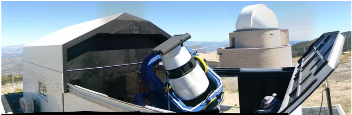
Fig. 1. Telescope Fabra ROA at Montsec (TFRM) at its current observing site, the Astronomical Observatory of Montsec (Catalonia, Spain). See reinforced glass-fiber enclosure with sliding roof open and South gable wall opening.
