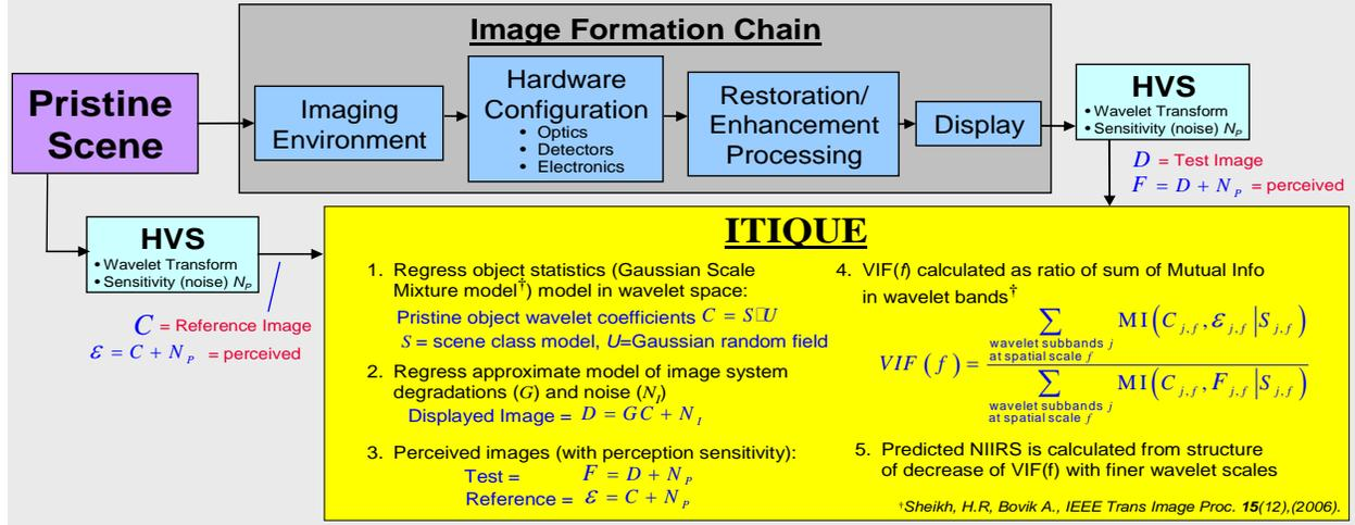
Fig. 4. ITIQUE framework uses VIF concept to measure perceptually relevant mutual information at several feature scale sizes and predict NIIRS
