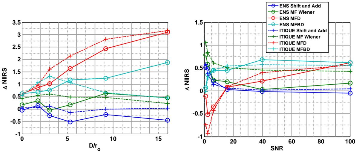
Fig. 8 plots the improvement gained by different image restoration algorithms over the raw imagery, illustrating the utility of ITIQUE as an analysis tool for system and algorithm design, optimization, comparison, and selection.
