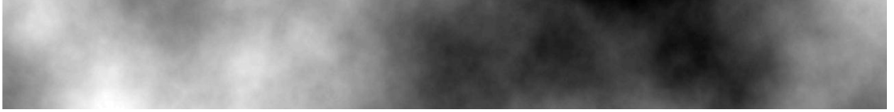
Fig. 3. Gray scale representation of phase screen corresponding to Tatarskii power spectrum with the outer scale L_0 that is seven fold longer than the phase screen width. The phase screen is generated using numerical grid with 8*512 \times 512 ( J=8 ) pixels.
