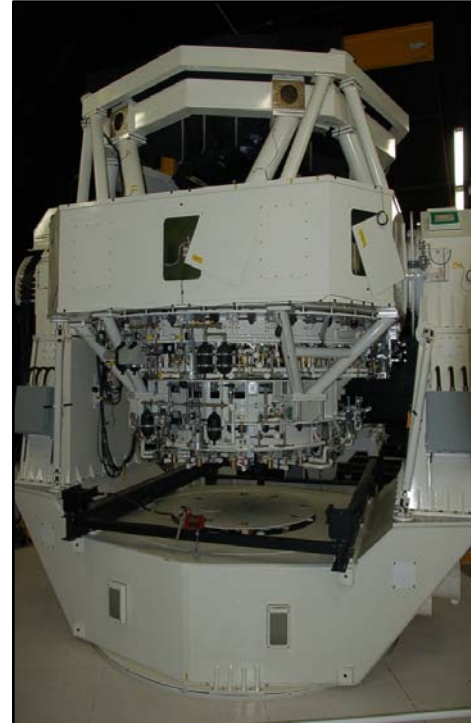
Figure 1: Two images of the Space Surveillance Telescope (SST). The telescope is a Mersenne-Schmidt system with powered primary, secondary, and tertiary mirrors. The compact layout achieved by the F/1.0 optics facilitates the mount gimbal's pointing performance.
