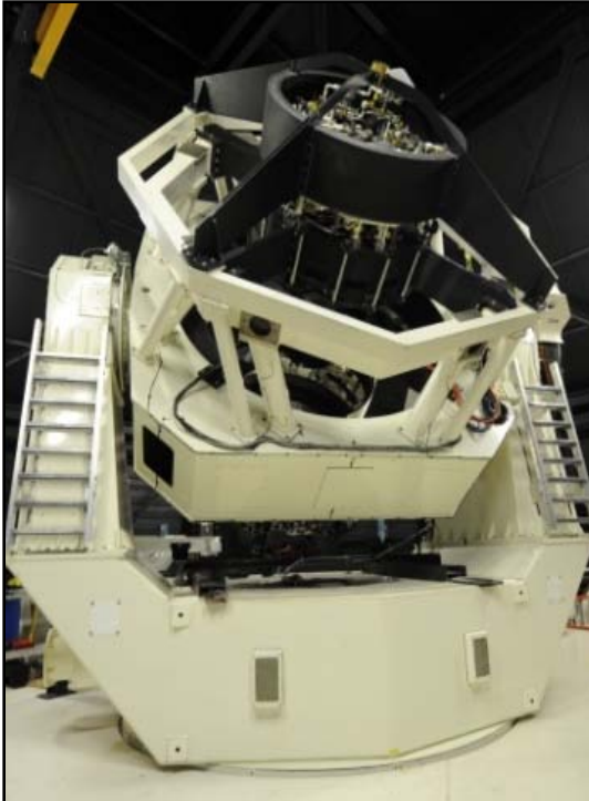
Figure 1: Two images of the Space Surveillance Telescope (SST). The telescope is a Mersenne-Schmidt system with powered primary, secondary, and tertiary mirrors. The compact layout achieved by the F/1.0 optics facilitates the mount gimbal's pointing performance.
