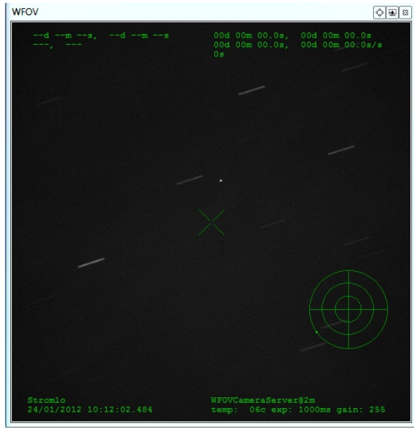
Fig. III: Picture of EOS Mt Stromlo Satellite Ranging System tracking object 21801 in front of the starfield.
