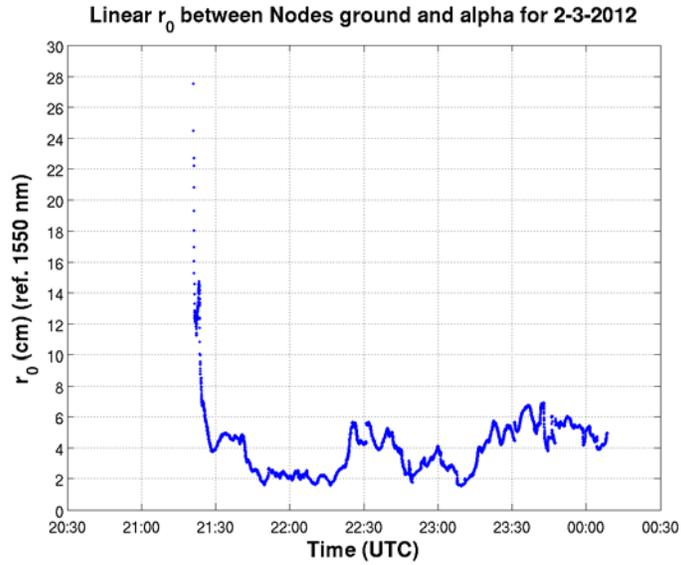
Figure 6 WRF-derived  $r_0$  for February 3, 2012 from Hollister to one of the aircraft.
