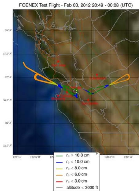
Figure 5 Values of  $r_0$  shown for each LOS between each communications node on February 3, 2012.
