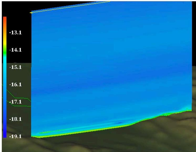
Figure 7 WRF-derived  $C_n^2$  in the area of Campbell, CA, on May 25, 2011. An elevated area of intense turbulence can be seen in the yellow colors a few hundred feet above the ground.
