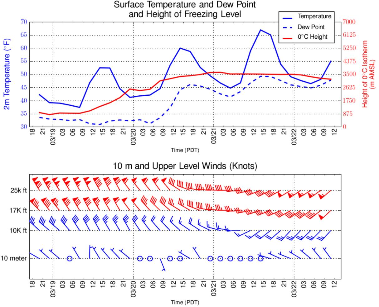
Figure 4 Forecasts of temperature, dew point temperature, 0° isotherm height (top) derived from the SREF ensemble forecast. Wind speed and direction are shown in the bottom plot at 10 meters above the surface, 10000, 17000, and 25000 feet above sea level.
