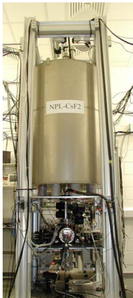
Figure 2: An atomic clock. Actually an atomic chronometer since it produces a continuous stream of uniform seconds but does not actually keep time. A chronometer becomes a clock when it is synchronized with Earth rotation, or, alternatively the Sun's passage through the sky, with noon at zenith.
