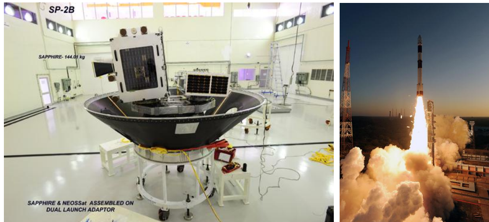
Fig.2. (Left) The Sapphire satellite (indicated) and NEOSSat (smaller satellite to Sapphire's right) mated to the PSLV dual launch adaptor. (Right): PSLV C20 launch (Image Credits: ISRO).
