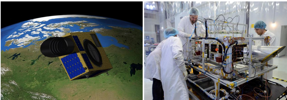
Fig.1. Left: The NEOSSat microsatellite artistic impression (Image Credit: University of Calgary). Right: NEOSSat being prepared for thermal environmental testing at the David Florida Laboratory in Ottawa, Ontario. The telescope baffle (beveled cylinder) is visible on the right. (Image Credit: Janice Lang, DRDC Ottawa).
