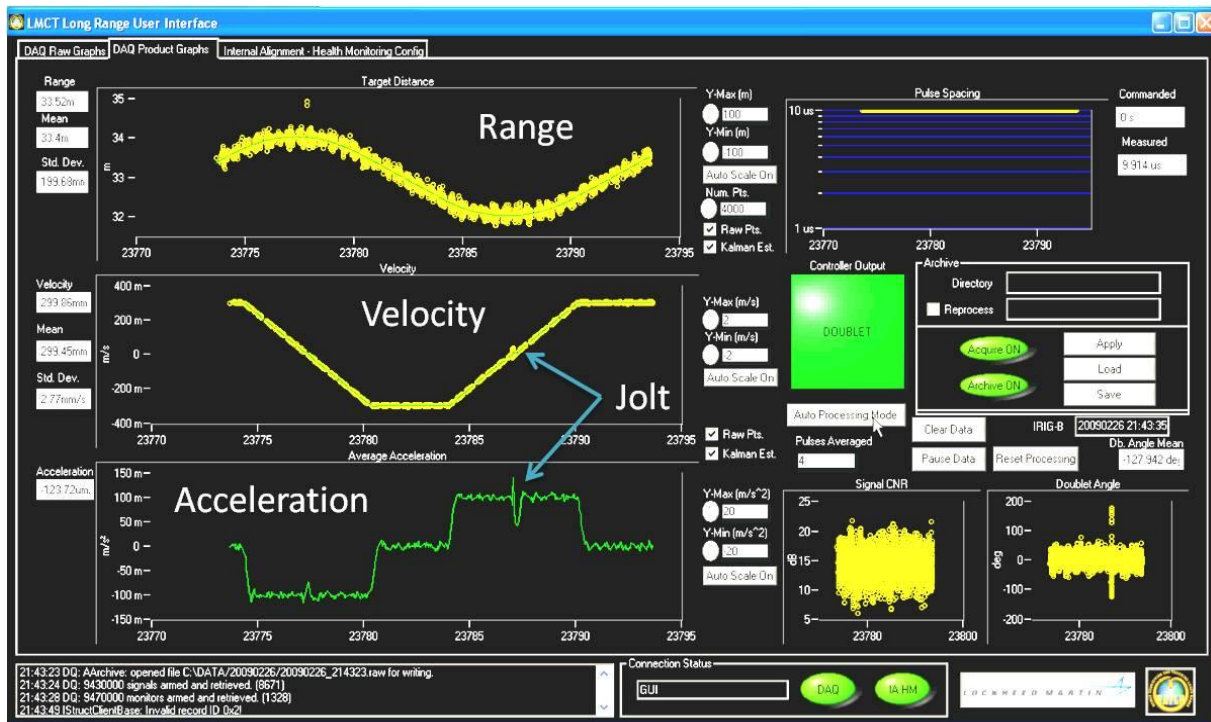
Figure 8. The coherent lidar system user interface illustrating track information. The lidar algorithm provides real-time range, velocity, and acceleration tracks as well as a number of other diagnostic signals. Note its ability to see acceleration jolts at the target turn-around points.
