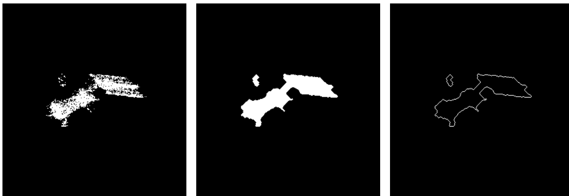
Fig. 2. Application of the shape extraction routine to the ISAR image presented in Fig. 1. Left: Gradient based watershed. Centre: Morphological filling. Right: Contour extraction.
