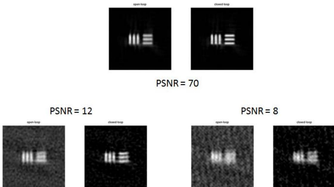
Figure 5 - Closing loop improves reconstructed imagery
