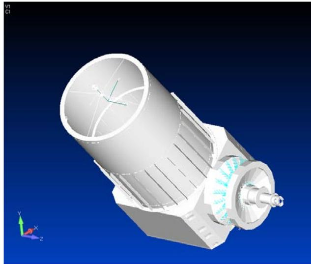
Fig. 2 – Finite element model of a large telescope with mechanically isolated probe beam
