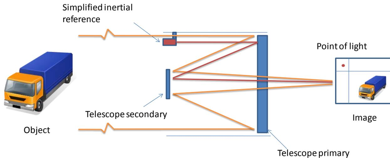
Figure 1 – Imaging system with simplified inertial reference
