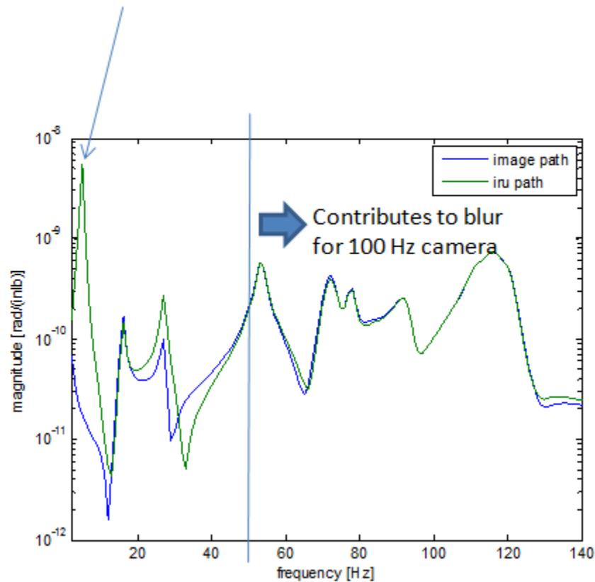
Figure 3 – Transfer functions generated from state space model
