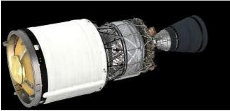
**Figure 1. Rendering of the Boeing Delta-IV Stage-2 upper stage rocket-body (from [11]).**
