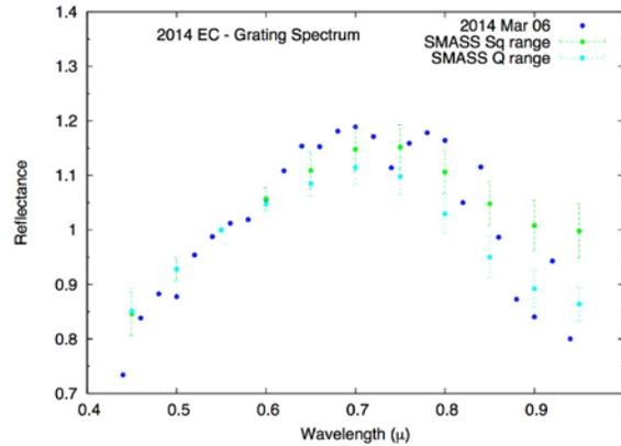
**Fig 9.** Spectrum of the NEO 2014 EC acquired using the simple grating system in the filter wheel of the MRO 2.4-meter telescope.
