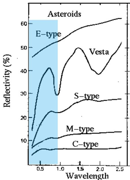
**Fig. 1.** Highlighted in blue is the wavelength range covered by the Magdalena Optical Spectroscopy System (MOSS), about 0.3 – 0.9 microns. Sample spectra for different asteroid taxonomic classes are shown. Even though this small range is not fully diagnostic (pairing it with IR spectra would be ideal), it is adequate to make first-order taxonomic identifications that lead to better constraints on albedo and thereby NEA size.
