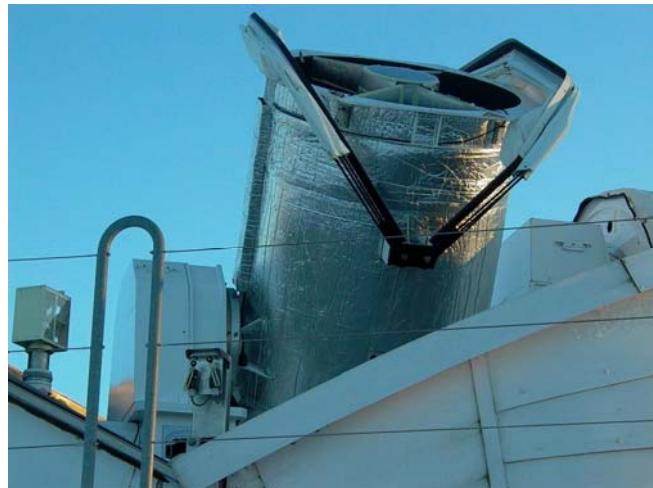
Figure 1: AIUB's 1-meter ZIMLAT telescope dedicated to the photometric and astrometric measurements.
