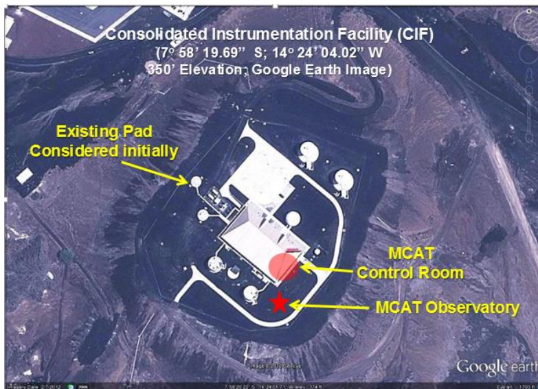
Fig. 3. Location of the MCAT Observatory. Steady trade winds prevailing from the SSE off the western coast of Africa ensure that a laminar airflow passes over MCAT before any turbulence forms from nearby buildings and structures.
