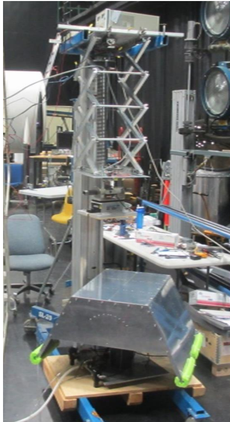
Figure 4. Reconfigurable Reactive Spacecraft (Orbital Object) Simulator
