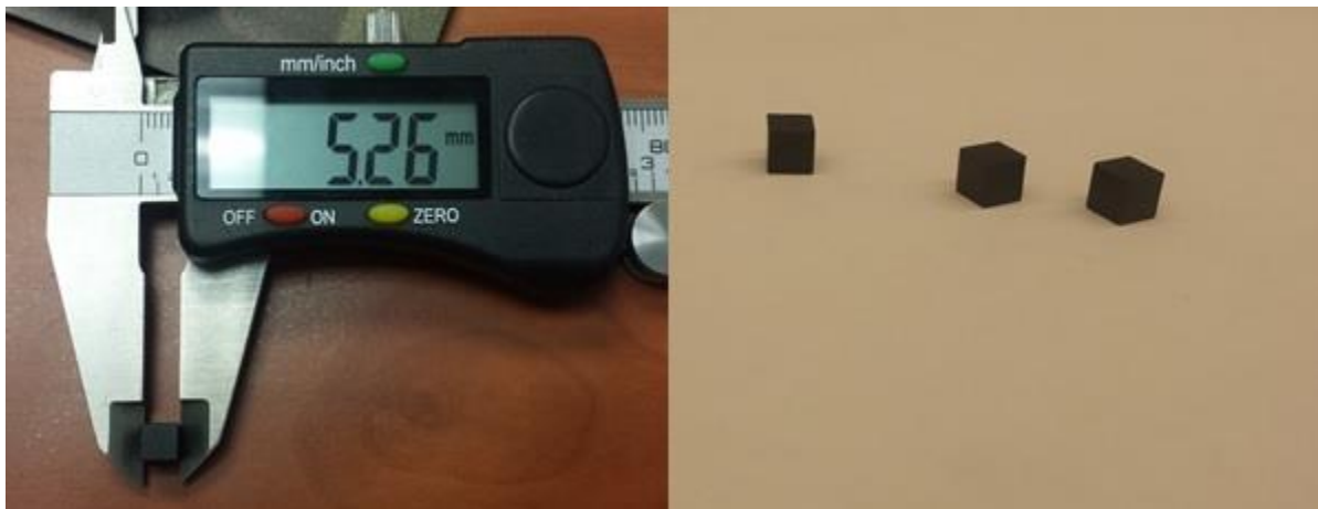
Fig. 8. Delrin (150SA) Samples Prepared for ASTM E 595 Test
