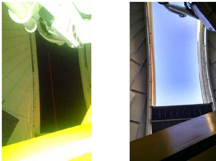
Fig. 3. (Left) The laser beam propagating to zenith through the slit of the Kuiper telescope dome is easily seen at night. (Right) Approximately the same view in daylight when the beam is very hard to see.
