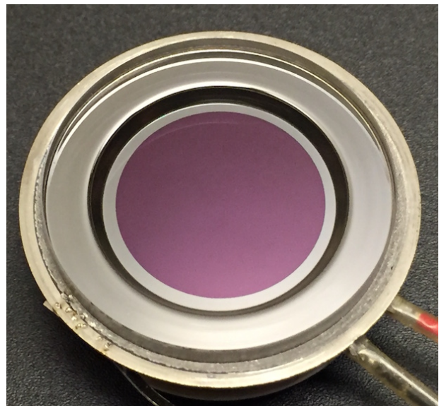
Fig. 4. A cross strip anode sealed tube sensor with a 22 mm readout anode, a pair of 6 \mu\text{m} pore 80:1 l/d MCPs and a Super-GenII photocathode.
