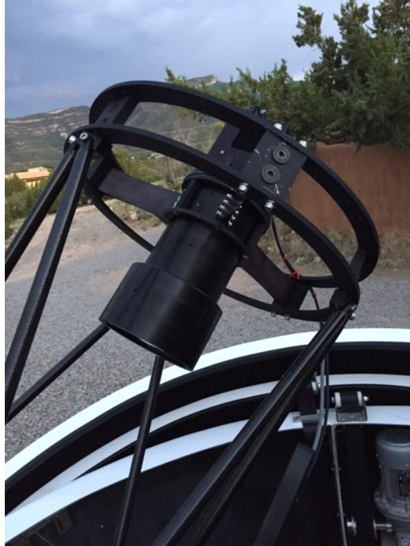
Fig. 5. Ackermann-designed prime focus focal reducer mounted on a C-14 with prime focus corrector plate removed. The pupil for this unique system is on the first corrector lens, not, as is usual, at the primary mirror. This system produces a 3.6^\circ \times 2.4^\circ FOV on a KAF16070 interline transfer CCD in a Finger Lakes Instruments camera.
