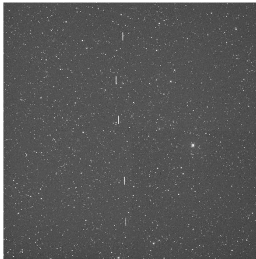
Fig. 3. The Stare-mode is designed to detect UCTs. Streak length is measured and, combined with exposure time, used to estimate the orbital altitude of the detected object (s). Thus, while searching for LEO was of prime interest in creating this mode, objects at any altitude could feasibly be detected.
