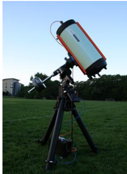
Fig. 1. The 11" Celestron RASA and Manta G-235 on a Losmandy G11 mount in Needham, MA before a night of observations.
