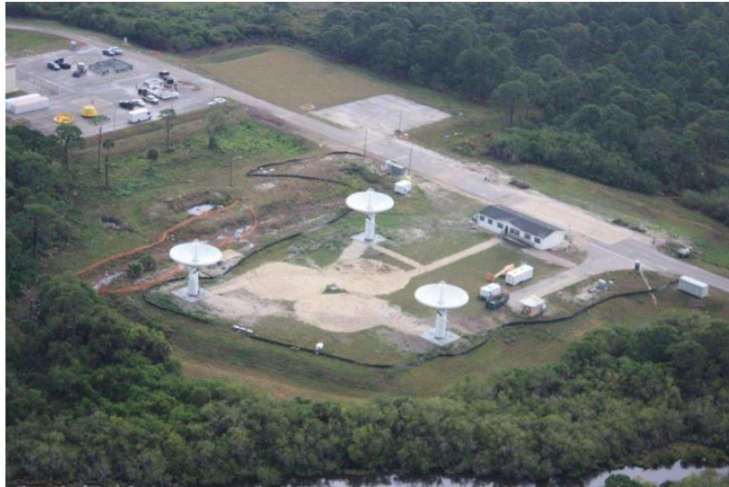
Fig. 4. Overhead shot of the KaBOOM site at the Kennedy Space Center. It is comprised of three 12m diameter antennas. The operations center is seen just to the right of center. Spacing between the antennas is 60m.
