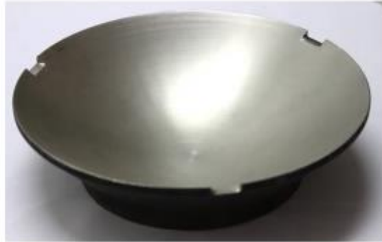
Fig. 18. 3D manufactured 30 cm antenna.
