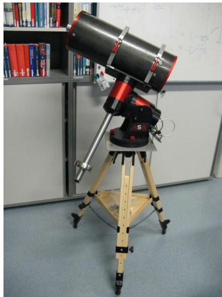
Fig. 1: Used equatorial telescope system with direct-drive telescope mount and 12" telescope mock-up.
