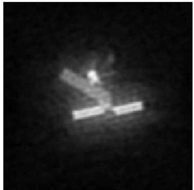
Figure 22. This is the Polak-Ribiere-Polyak constrained by Fletcher-Reeves case. After 1100 function evaluations this method appears almost as detailed as LBFGSB case at 500 function evaluations.
