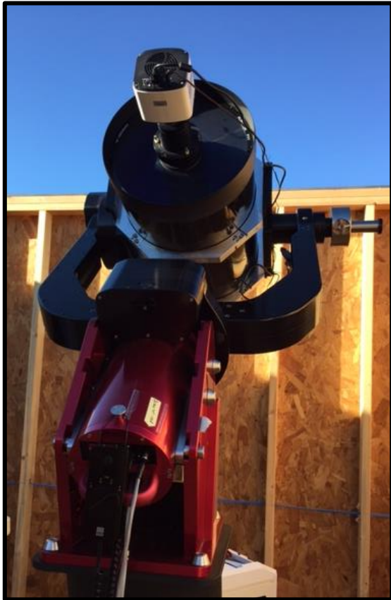
Fig. 2 – This 0.35m optical system is currently deployed at JTMA's R&D site just outside of Albuquerque, NM. The system is based upon a 14" Celestron SCT with a Hyperstar prime focus corrector.
