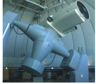
(c) The 1 m Optical Ground Station (OGS) telescope in the Teide Observatory. Credits: ESA
