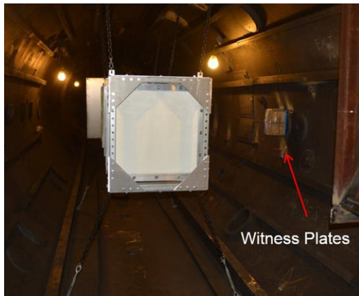
Fig. 3. Pre Preshot target hanging in AEDC vacuum chamber looking down range. Witness plate assembly was mounted on the side of the chamber facing the target (Left). Target post-test looking down range. The fifth bumper shield is lying on the floor of the chamber (Right). Images by AEDC.
