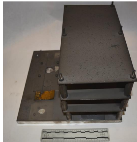
Fig. 1. Pre Preshot target with seven bumper shields being loaded into the AEDC test chamber. Projectile entry was from left to right.
