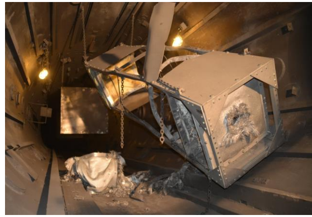
Fig. 3. Pre Preshot target hanging in AEDC vacuum chamber looking down range. Witness plate assembly was mounted on the side of the chamber facing the target (Left). Target post-test looking down range. The fifth bumper shield is lying on the floor of the chamber (Right). Images by AEDC.
