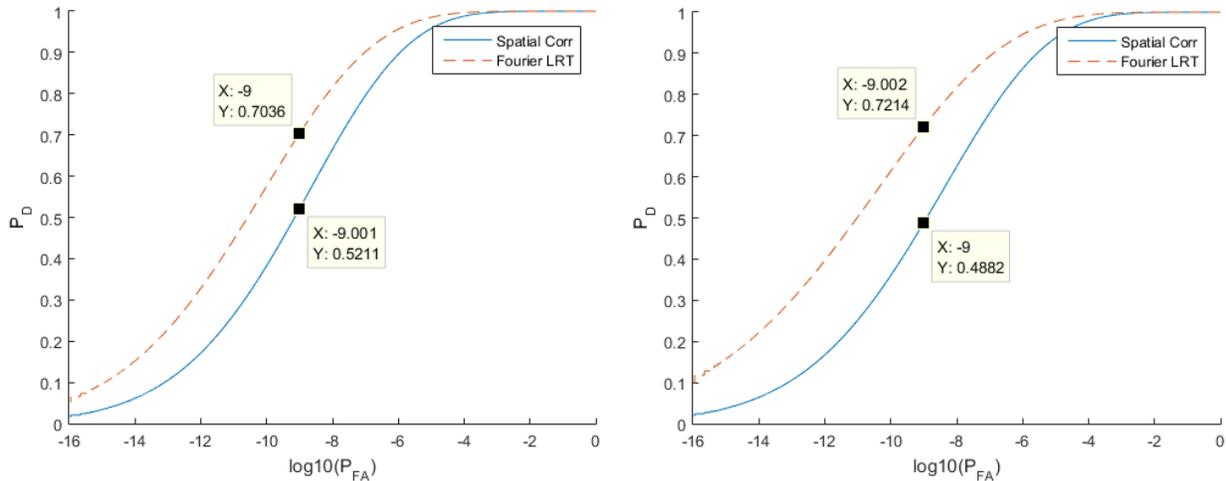
Fig. 5: ROC curve for the matched filter and Fourier LRT methods. Scenario 1,  $D/r_0 = 5$  (left). Scenario 2,  $D/r_0 = 3$  (right).
