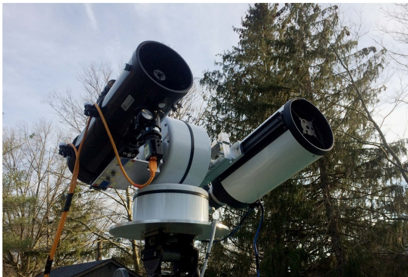
Fig. 1. Photograph of the prototype slitless spectrometer installed on a tracking mount
