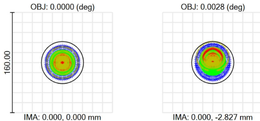
Fig. 4: Spot diagram produced at imaging camera over wavelength range 800 - 950 nm. Left: On-axis field. Right: 10" off-axis field.
