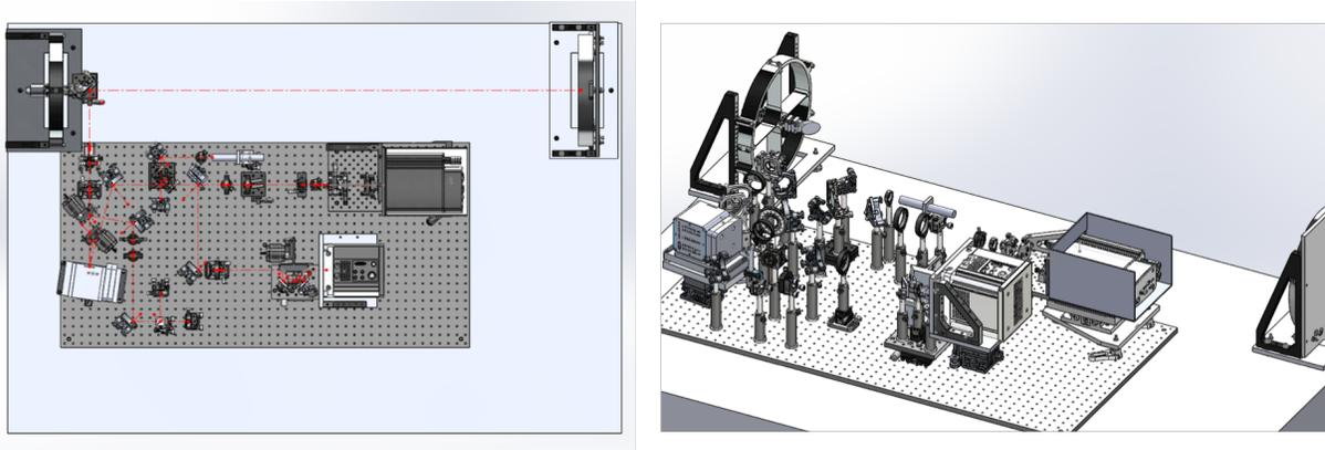
Fig. 5: Mechanical layout of AOI. Left: Top view of the mechanical layout. Right: Trimetric view of the mechanical layout
