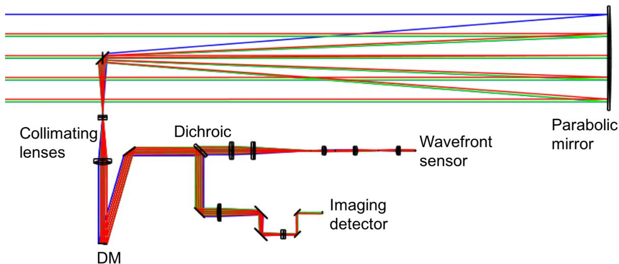
Fig. 3: Layout of the AOI system. The parabolic mirror focusses the beam which is collimated to the DM pupil size by two lenses. After reflecting off the DM light is split by the dichroic between the wavefront sensor and imaging arm.
