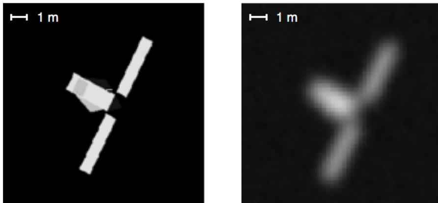
Fig. 1: Left: Ideal image of an iridium satellite. Right: Simulated image of satellite through AOI. The image is an  $50 \times 50$  pixel area of the detector.
