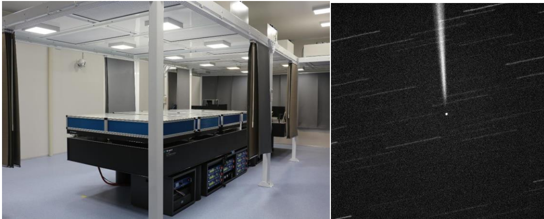
Fig 5: Left, Modularized laser in Learmonth Clean Room. Right: Laser tracking a MEO Satellite
