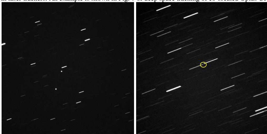
Fig 7: Left Tracking Optics C1 & D3 in GEO. Right a faint target detected amongst star clutter
