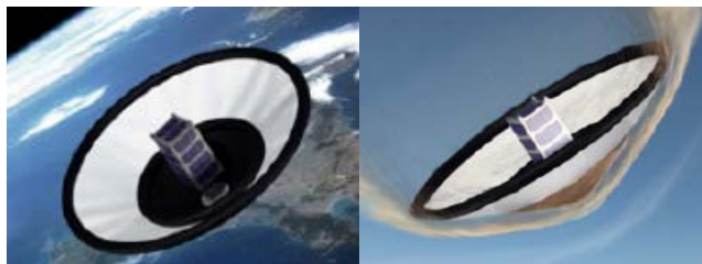
Fig. 3. Proposed d2U CubeSat DRS mechanism [10]
