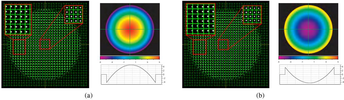
Fig. 2. Example of Hartmanngram and reconstructed wavefront – positive and negative defocus.
