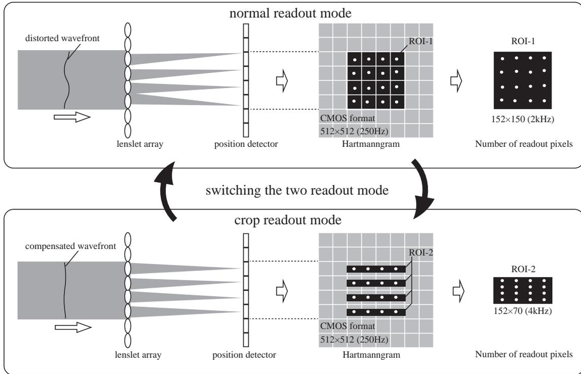
Fig. 9. Two typical operation modes: normal readout mode and crop readout mode.
