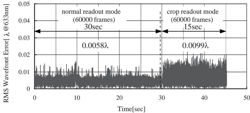
Fig. 10. RMS wavefront error with different operation mode.
