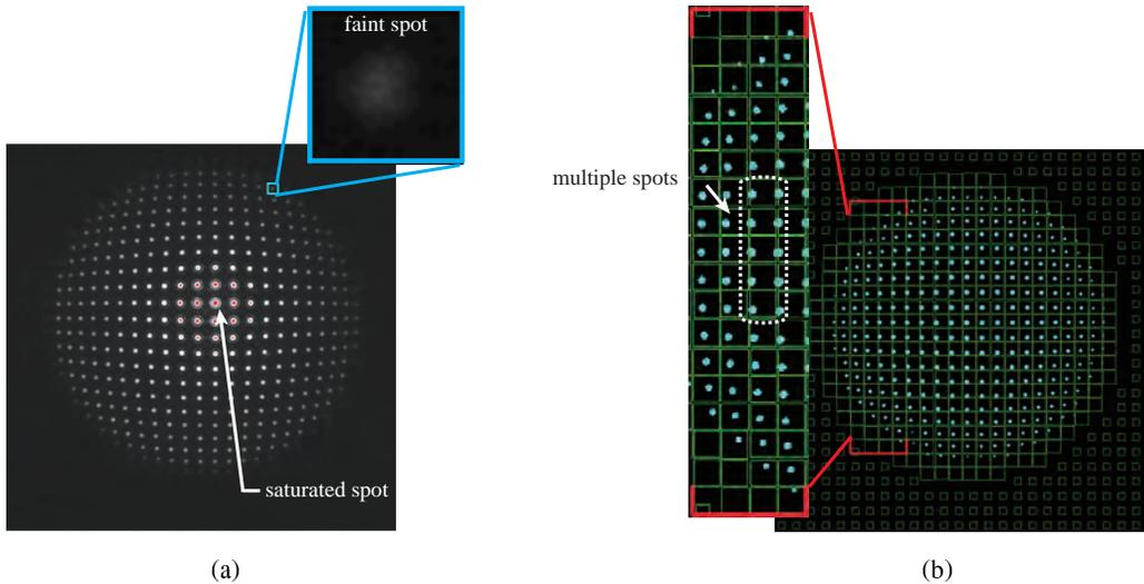
Fig. 3. Example of Hartmanngram – (a) non-uniform illuminance distribution, (b) multiple spots.
