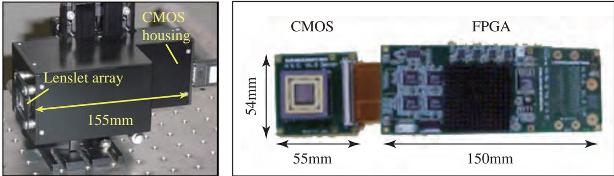
Fig. 8. High-frame rate SHWFS – (a) outside appearance, (b) circuit board.
