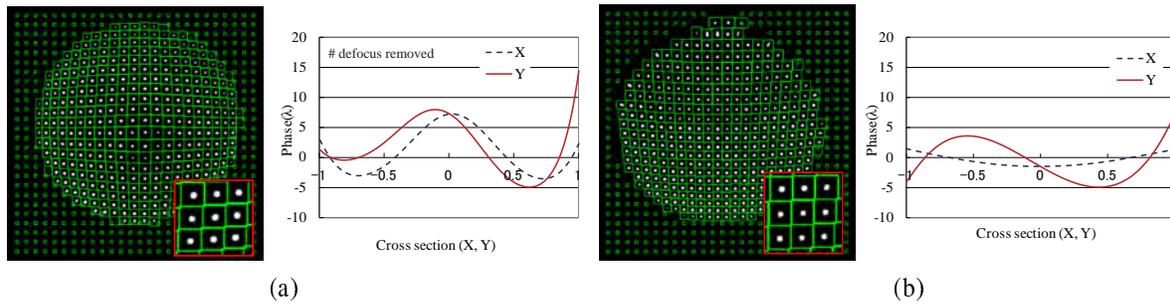
Fig. 6. Example of Hartmanngram with the related centroid areas for highly aberrated wavefront.
