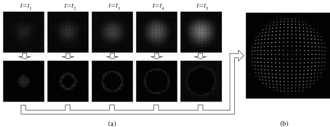
Fig. 4. Hartmanngram combined with different exposure frames.
