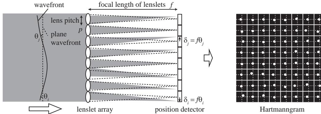
Fig. 1. Principle of Shack-Hartmann wavefront sensing technique
