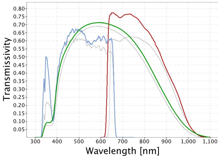
Fig. 3. The Gaia passband system. The colored lines represent the modified passbands that are representative of the colors released in DR2. The G-band curve is shown in green, the  $G_{BP}$  in blue, and the  $G_{RP}$  in red. The grey lines are the pre-launch estimations for the passbands.
