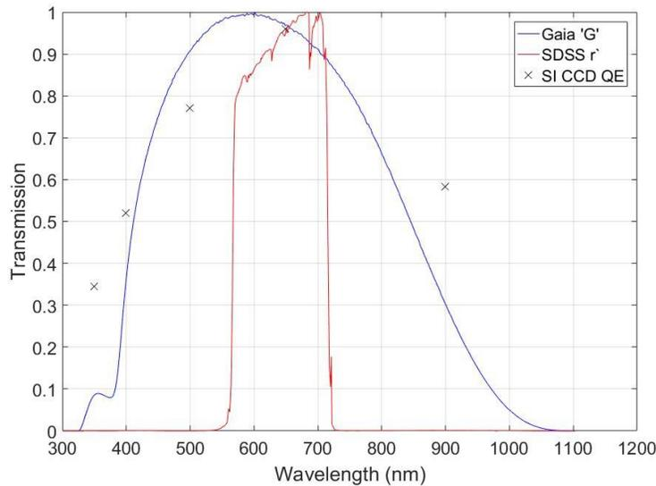
Fig. 2. The Gaia G-band transmission curve as compared to the SDSS  $r'$  filter and the quantum efficiency of a typical E2V Charged Coupled Device.
