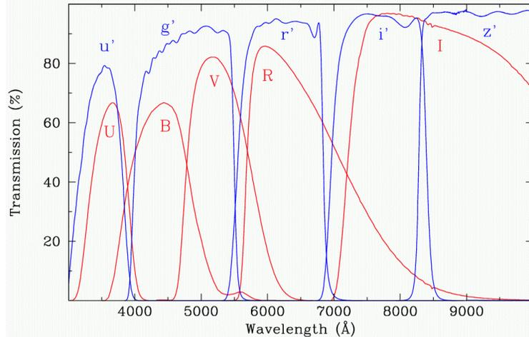
Fig. 2. Filter transmission curves for the Johnson-Bessel and the Sloan Digital Sky Survey filter system.
