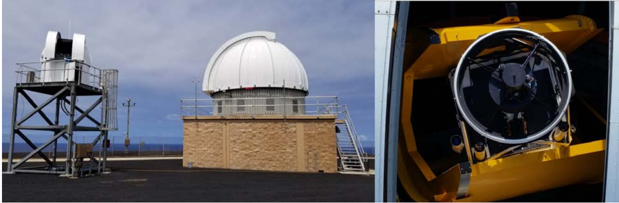
Fig. 1. ES-MCAT on Ascension Island. Left: The John Africano Observatory comprises the 1.3m ES-MCAT telescope, the 0.4m Officina Stellare telescope (on the platform to the left of MCAT in the newly installed 2.5m Observa-Dome), and is monitored by a suite of weather sensors (mast between telescopes). Right: The 1.3m f/4 DFM telescope is designed to track directly through the zenith at Ascension Island’s low latitude location ( 7^{\circ} 58' S, 14^{\circ} 24' ).
