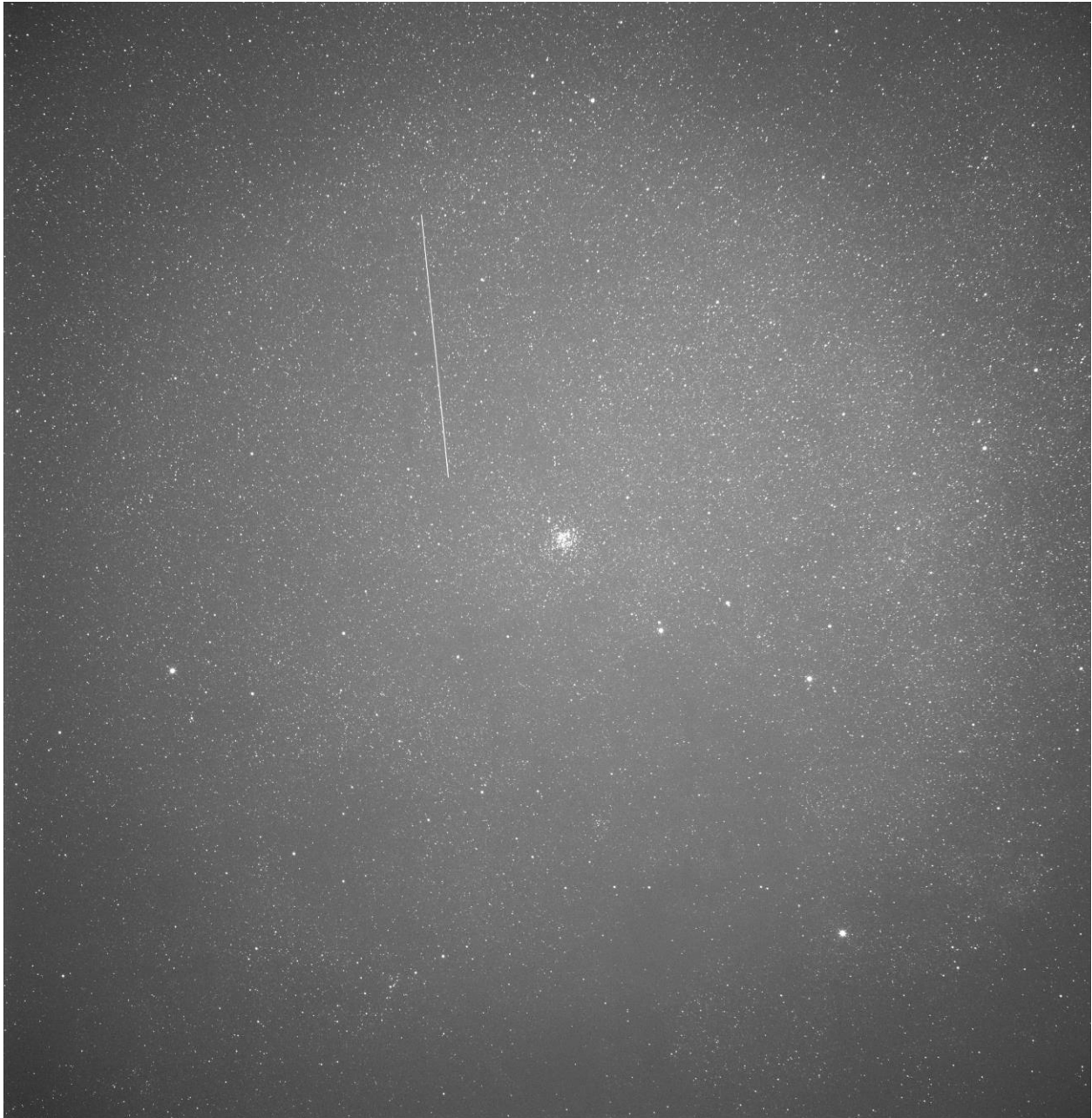
Figure 1. Low earth satellite streak across a typical Pomenis frame. The full 36.7×36.7 mm (51.9 mm diagonal) Apogee Alta F9000 camera format size is show, uncorrected for the slight vignetting of the field of view beyond about 44 mm.
