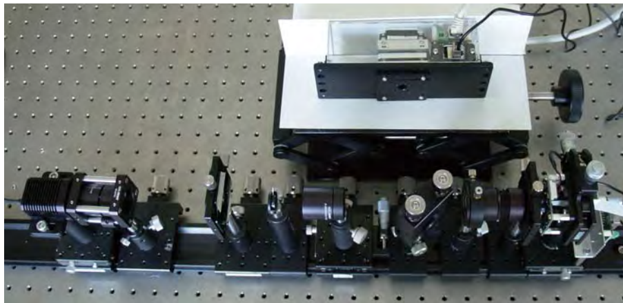
Fig. 16: Prototype model of extended scene SH-WFS for onboard satellite.
