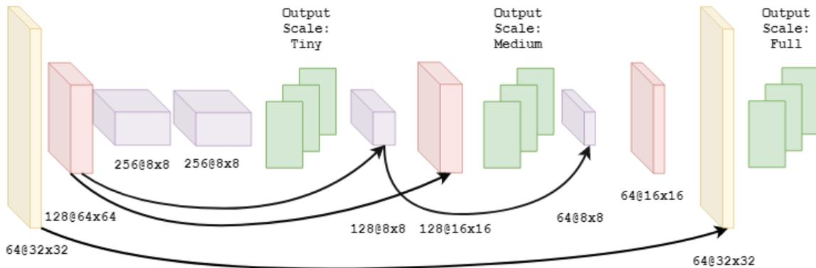
**Figure 4. Multiscale Architecture for Small Objects**
