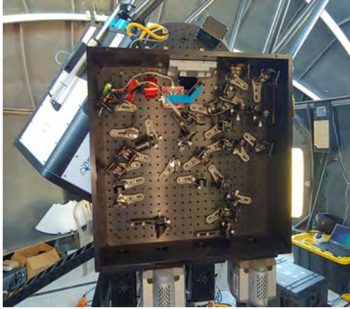
Fig. 1: The QWSSI instrument mounted on NPOI PW1000-1, for first light on Jun 8, 2020 .
