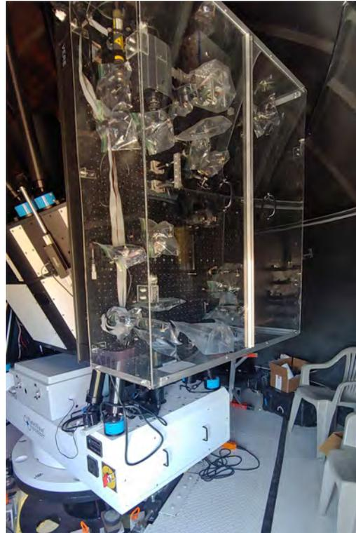
Fig. 4: Adaptive Optics breadboard # 1 (AO-1) mounted on a Nasmyth port for PW1000-1 at NPOI.
