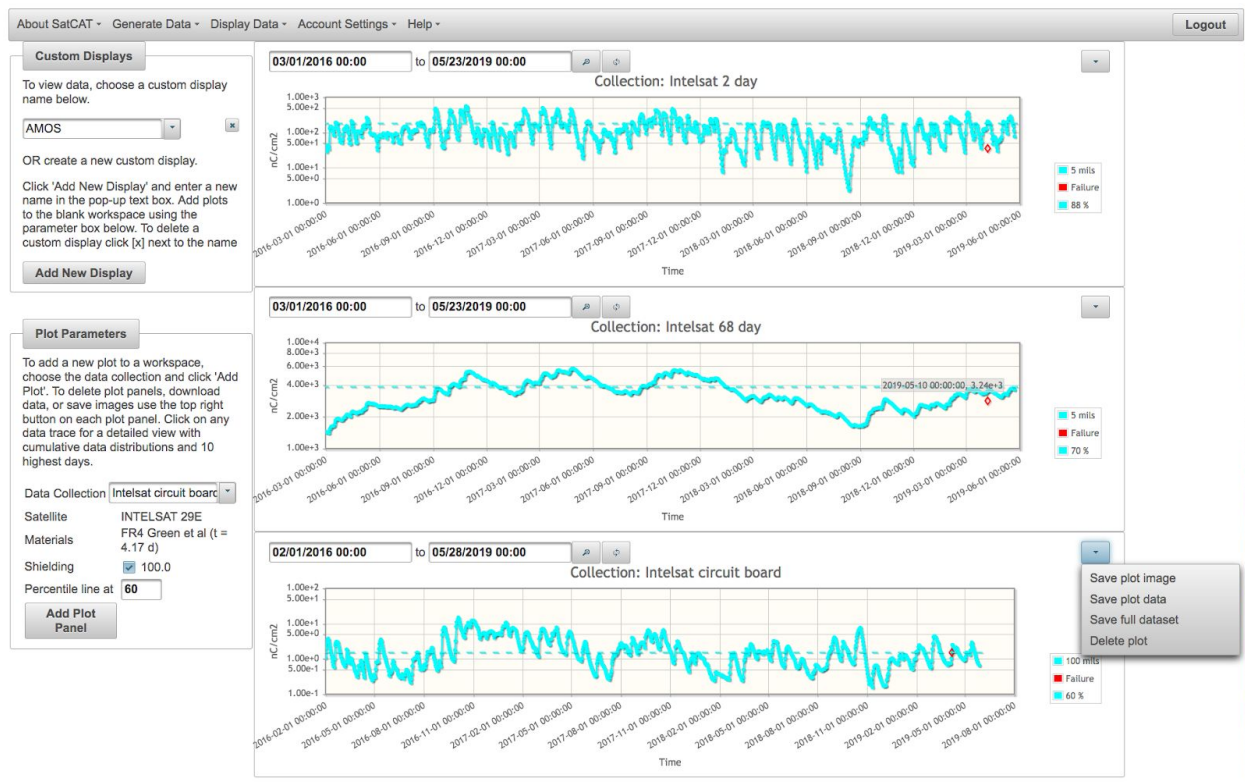
Fig 1. Demonstration of the SatCAT application showing the expected accumulated charge in three different types of components. The top panel shows the charge expected to accumulate in a lightly shielded generic Teflon cable. The middle panel shows the charge expected to accumulate in a lightly shielded Teflon FEP cable. The bottom panel shows the charge expected to accumulate in a deeply embedded FR4 circuit board. The red diamond marks the approximate time of the Intelsat 29E failure. The dashed lines show the percentile level of the accumulated charge at the time of the anomaly. For example, the 88 percentile line is drawn on the top panel. The accumulated charge was below this level for 88% of the mission and was above this level for only 22% of the mission.
