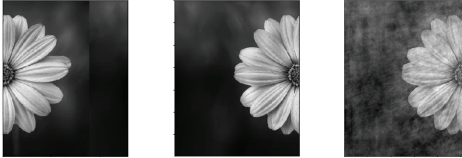
Figure 1 The phase from the Fourier transform of the right hand half of the flower is combined with the amplitude from the left hand half, and then the inverse transform of the combination is shown on the right. As imaging is essentially a Fourier transform process, this demonstration motivates us to investigate new ways to compensate for phase distortions, or infer them in a more robust way.
