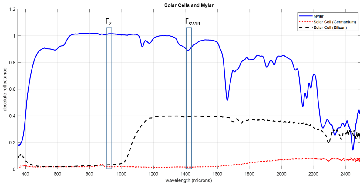
Fig 9: Reflectance for Solar Cell Materials (Germanium and Silicon) and Mylar – Discriminator filters placed at chosen observation wavelengths.
