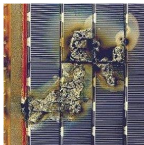
Fig. 6. Impact of ESDs on solar panels [19]
