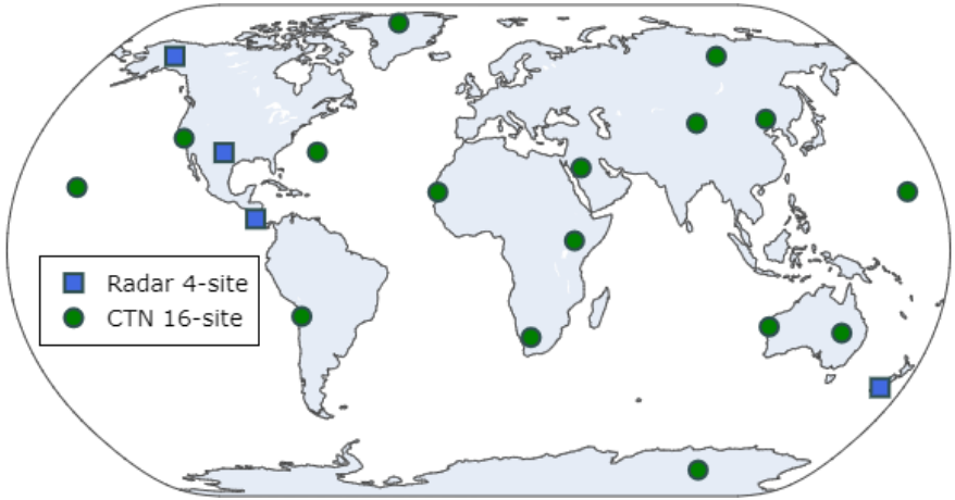
Figure 7. Hypothetical sensor laydown for simulation: sixteen cathemeral telescope sites and four radar sites.
