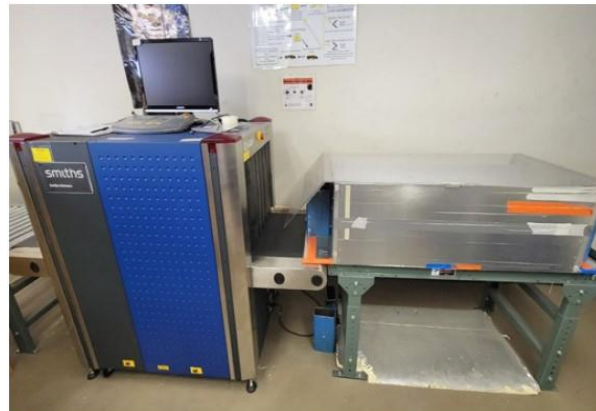
Figure 3. Hi-Scan 6046si X-ray scanner with added rollers and shoe.
