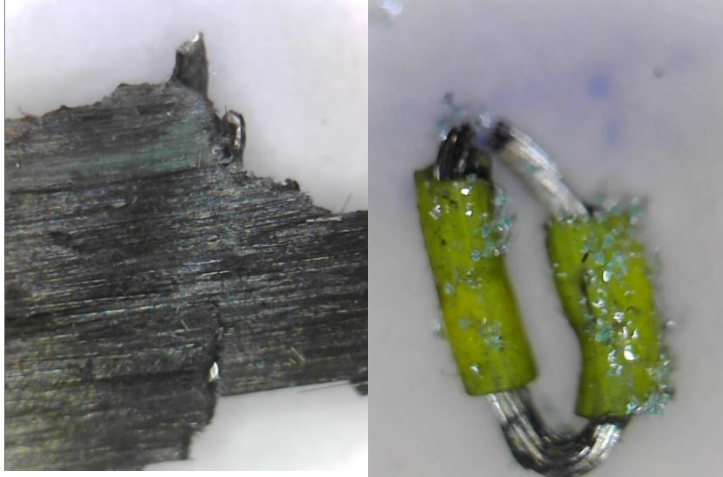
Figure 6. CFRP with epoxy and metal (left); copper wire with plastic insulation (right)
