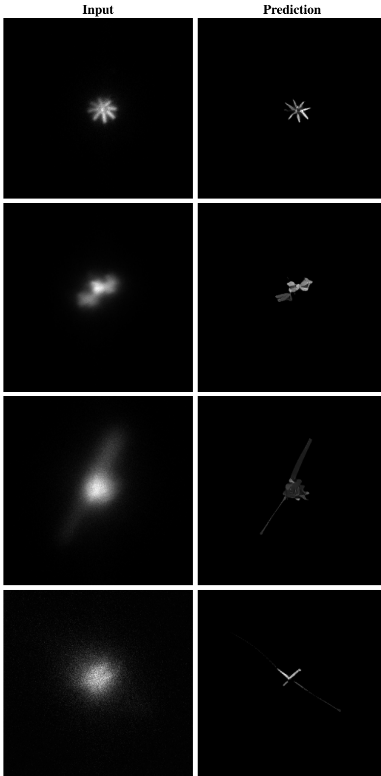
Fig. 11: Visual results of custom Real-ESRGAN model on real-world data. Rows 1, 2, 3, and 4 show the image restorations of Cosmos 1803, Cosmos 2084, Meteor-M 2, and Starlink-3558.
